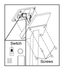
to change the unit of measurement. Reattach the console with the four screws. **Be careful not to pinch** any of the wires.
